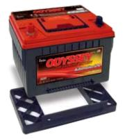
Optional height adapter may be used on the 34-PC1500 for installations where a group 24 or group 27 is required. Snap the adapter securely into place on the bottom of the 34-PC1500 battery. In some installations, a 34-PC1500 with this adapter may be used to replace a group 24F or 27F depending on required cable length.
